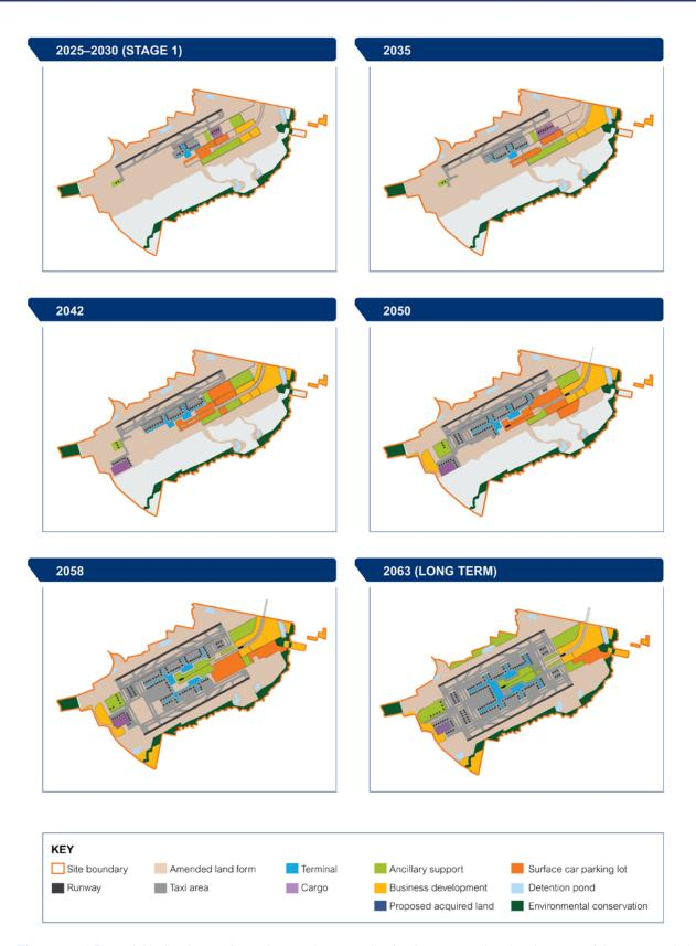
Figure 30–1 Potential indicative configurations and sequencing for the progressive development of the proposed airport
